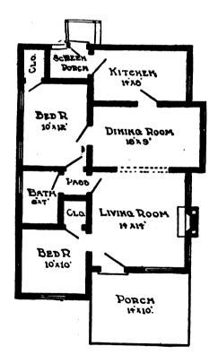
Fig. 92.—COMMUNITY I. PICTURE AND PLAN OF MILL-CUT BUNGALOW OF 5 ROOMS AND CELLAR.
